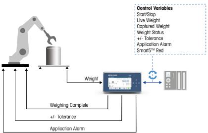
This setup demonstrates a self-contained, weight-based sorting machine. Higher-level systems such as PLCs or PCs read the result from the IND360.
