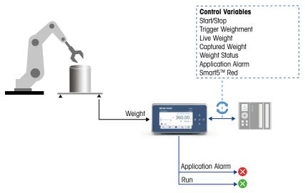
The PLC sends a command to trigger the weight capture as soon as the item has been placed. The resulting captured weight and status information are available on the PLC network once the weightment is completed.
