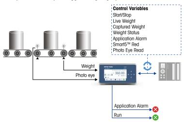
The two photo eyes that trigger the weighing operation are directly connected to the input of IND360. This method provides the best reaction time, least jitter and saves I/O space on the PLC. The live weight and photo eye status are continuously transmitted to the PLC. The resulting captured weight and status information are sent to the PLC once a weighing transaction is completed.
