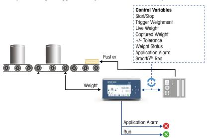
The PLC sends a command to trigger the weight capture. The IND360 monitors the weight tolerance and signals the PLC when the item must be rejected via a discrete signal or via Boolean value transmitted to the PLC. Each weight transaction includes measurement value, tolerances, and checkweighing data in addition to live weight data that can be read at any time.
