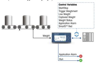
The PLC sends a command to trigger the weight capture in a similar way as if there were photo eyes installed. This operating mode avoids the need for photo eyes, which simplifies hygienic design but requires that the PLC knows the position of the item. The live weight is continuously transmitted to the PLC, and the resulting captured weight and status information are sent to the PLC once the weighment is completed.
