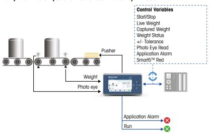
Two photo eyes that trigger the weighing operation and the reject pushers are directly connected to the inputs and outputs of IND360. This method provides the best reaction time, least jitter, and saves I/O space on the PLC. Live weight and photo eye status are continuously transmitted to the PLC. On completion of a weight capture, the resulting captured weight, tolerance, and status information are available to the PLC.
