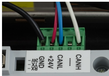
Figure 2-78: PowerMount Cable Connection to Main Board
