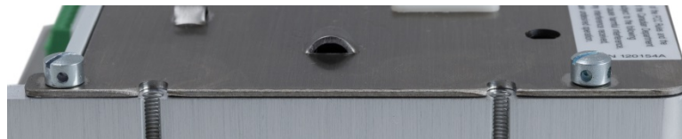
Figure 2-127: Sealing Screws Installed
