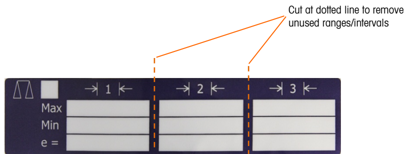
Figure 2-124: Preparing the Capacity Label
