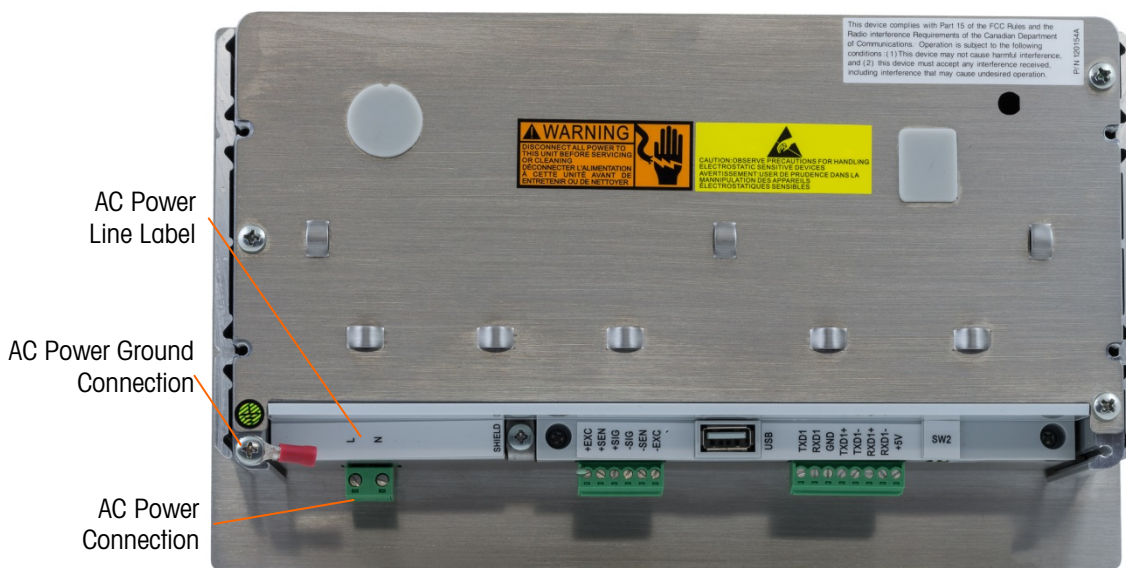
Figure 2-29: AC Power Connection on Panel Mount
