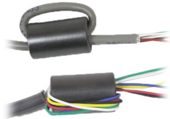
Figure 2-20: Installing the Ferrite Cores
