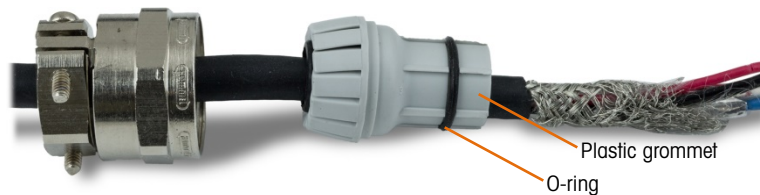
Figure 2-70: Cable Gland Installed on Cable
